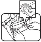
2. Pull the metal rod towards you, while the safety lock release buttons are being pressed. This will unlock the metal rod from the safety locks, allowing the legs to fold into the desired position.
